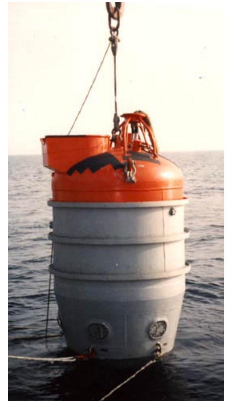
SRC-8 going up and over. Likely, the last time any SRC will see 850 fsw. The SRC is required to dive to test depth following a major overhaul.
