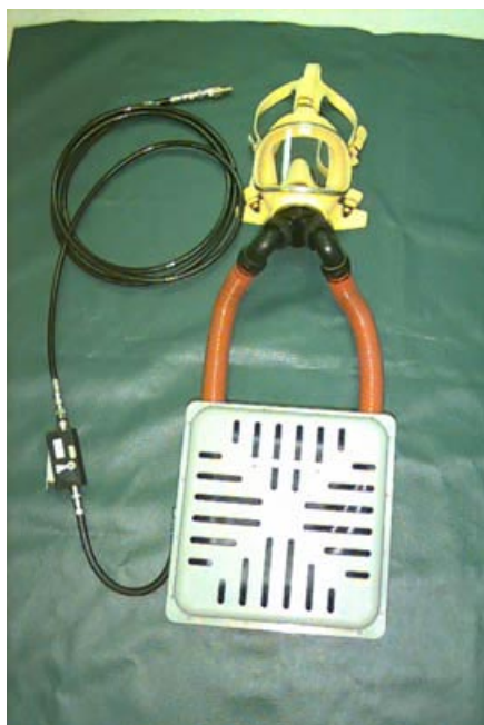
MK 18 MOD 1 EBA: Full face mask, breathing hoses, C control block with hose whip for gas supply.
